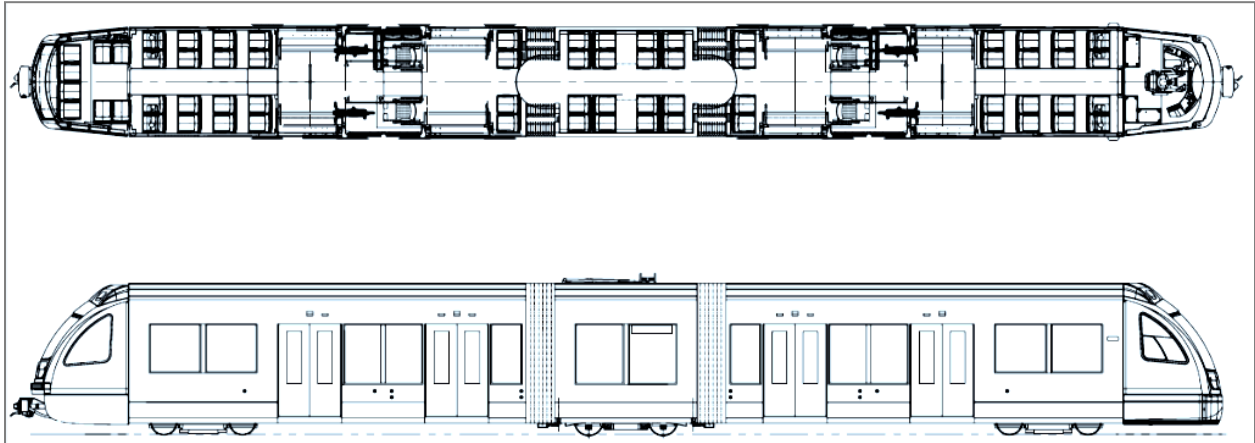
Figure 2-27: Seat and Door Arrangement of a Light Rail Vehicle Currently in Operation in Portland, Oregon
