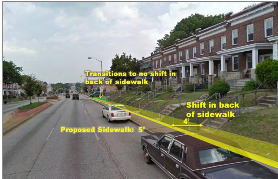
Example of proposed right-of-way within Allendale-West Mulberry Historic District/Keilty Daylight Rowhouse Historic District at Gwynns Falls
